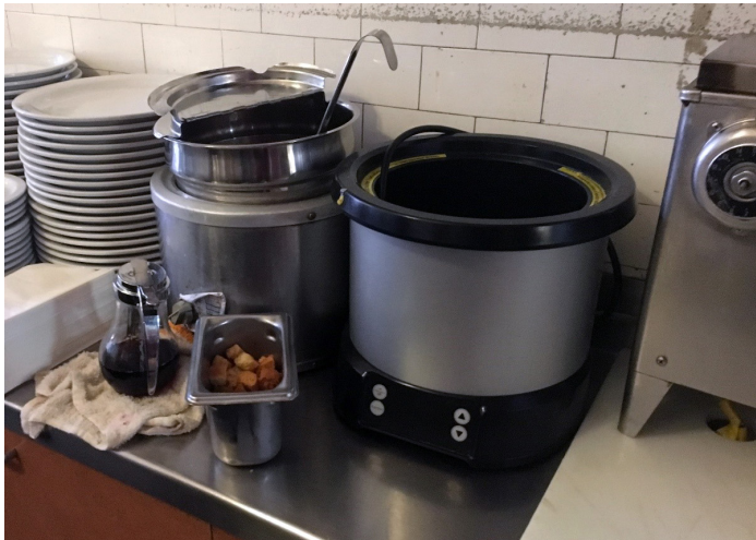
Original wet-well soup warmer (left) alongside the replacement induction dry-well soup warmer (right).
