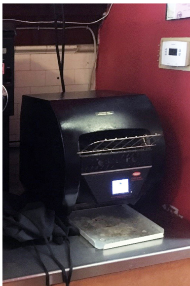
Replacement conveyor toaster with programmable controls and energy setback mode.
