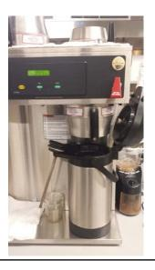
Coffee brewer with built-in logic for energy saving mode. After 4 hour from last done brewing, the thermostat heater for water reduce temperature set-point.
