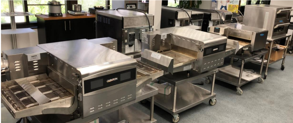
Figure 1: Hot Air Impingement Rapid Cook Ovens
