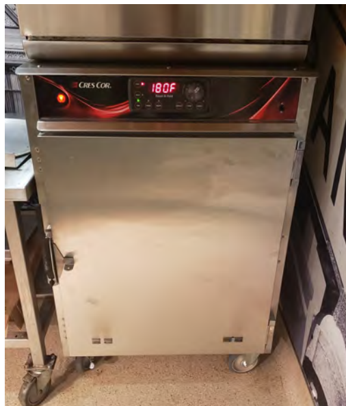
Figure 24: Site B Replacement Cook and Hold Oven
