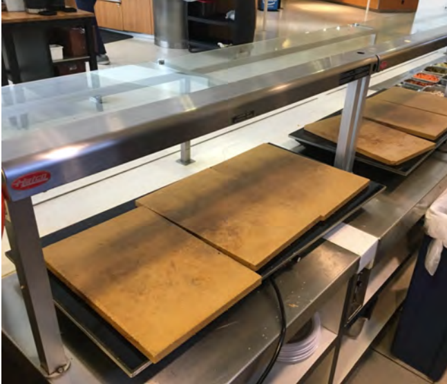
Figure 8: Two Heated Shelves with Pizza Stones and Overhead Heat Lamps
