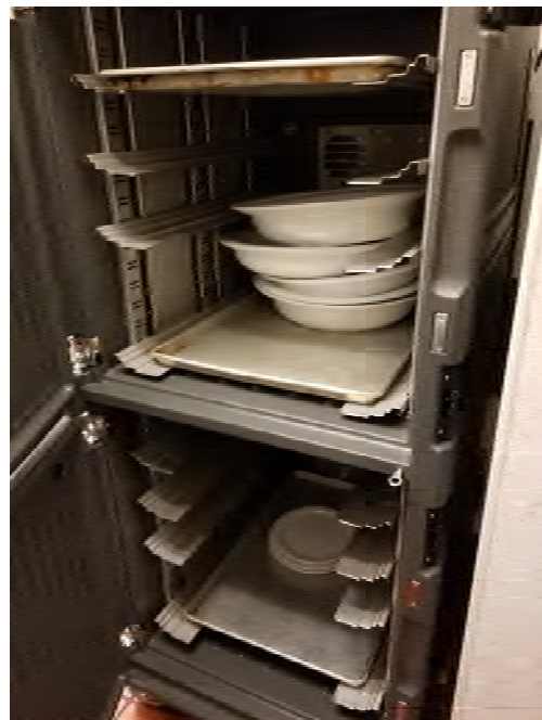
Figure 70: Replacement Dual Compartment Holding Cabinet, Only Top Compartment Heated
