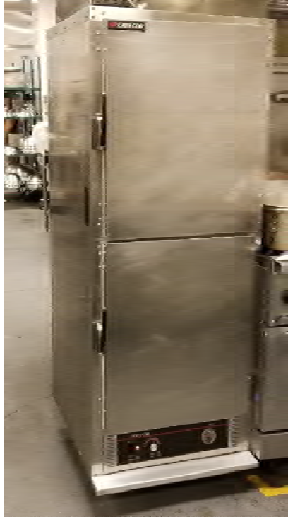
Figure 17: Baseline Holding Cabinet
